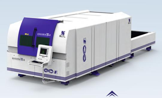
2D Cutting with Enclosure & Pallet Changer
